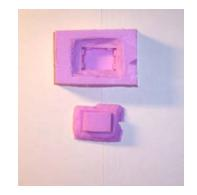
resin then insert the plug, making sure it's all the way down into the hole. This forces the excess resin to ooze up out of the hole and overflow the edges of your plug insuring that your wall sections are all totally filled. Once cured, you remove the plug and voila! There is your complete casting. The pictures of my two piece cupola mold show you how the mold looks when done (it has a "vee" notch on the top and bottom to show which ends go together).
